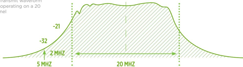
The plot shows that the energy is concentrated within the channel of operation, but there is some energy within the adjacent frequencies. Within 2 MHz of the channel edge, the transmit signal is approximately 21 dB lower. At 5 MHz, the transmit signal is approximately 32 dB lower. In the case of
