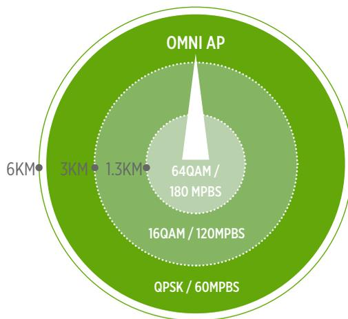
Omni antennas have lower gain than sector antennas and so the ranges for the higher modulations are shorter. A typical omni antenna may have 6 dB of lower gain than a sector antenna. This has the effect of halving the range of each of the modulations, which can impact Area Average Capacity. An AP with an omni antenna configured with a 40 MHz channel has Area Average Capacity of 69 Mbps.
