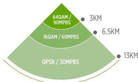
In the coverage area shown above, the location of the subscriber modules (SMs) defines how much capacity can be delivered from the access point. If all the SMs are located within the 64QAM coverage area, then the AP has the capacity to deliver 90 Mbps. If all the SMs are located within the QPSK coverage area, then the AP has the capacity to deliver 30 Mbps. If the SMs are distributed across the different coverage areas, then the capacity
